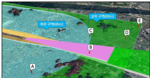
Fig. 7. Location within straight-in instrument approach surface
