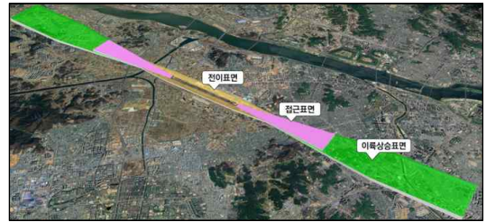
Fig. 3. Diagram of OFS at Gimpo Airport
