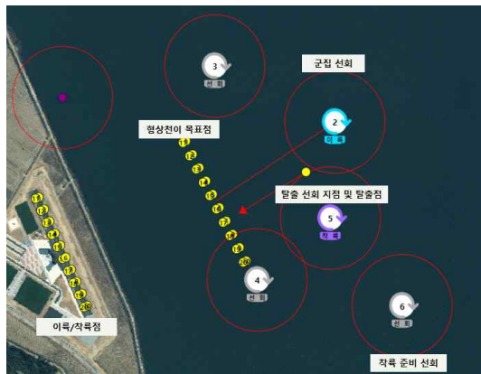
Fig. 7. Overall operational scenario for VTOL UAV swarm flight
